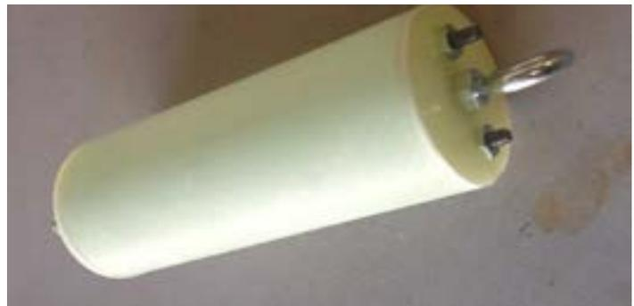
□ Step 5 - Mark the longer coupler 3.5" from the end with the double bulkplate that didn't have thread lock on the nuts. This will be the exposed part of the coupler. The single bulkplate with thread lock will be the covered part of the coupler that will go inside the payload section. Test fit the coupler inside the shorter payload tube and sand the single bulkplate if necessary.
