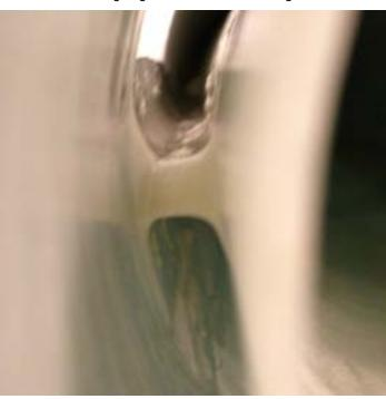
Step 25 - Use the same epoxy consistency to form fillets on the outside fin/body tube joint.
