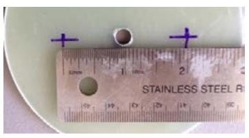
☐ Step 12 - Stack the 2 large bulkplates and 2 smaller bulkplates and temporarily secure the plates with a single eyebolt to hold them together. Drill through all 4 bulkplates at the points you just marked with a 1/4" drill bit.
