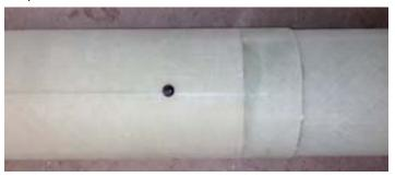
☐ Step 17 - Sand the outside of the motor tube to rough up the surface for the epoxy to stick to.
