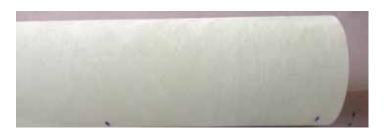
☐ Step 19 - Sand the slotted main body tube for at least 1/2" around the fin slots inside and outside to rough the surface for the fin fillets. Also sand where the centering rings will attach in front of the fin slots on the inside. You can wrap sand paper around a large dowel to help sand the inside of the body tube.
