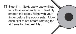
☐ Step 12 - It is also a good idea to CA the sharp tips of the fins to keep them from splintering on hard landings.
