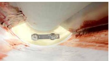
☐ Step 12 - Use the same epoxy consistency to form fillets on the outside fin/body tube joint.
