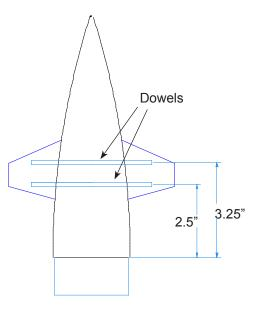
part that will hold the fin in place. The epoxy fillets only serve to fill any gaps for painting.
