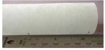
□ Step 13 - Sand the slotted main body tube for at least 1/2" around the fin slots inside and outside to rough the surface for the fin fillets. Also sand where the centering rings will attach in front of the fin slots on the inside. You can wrap sand paper around a large dowel to help sand the inside of the body tube.
