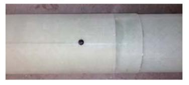
□ Step 7 - Sand the outside end of the coupler and the inside of the nose cone where the coupler and nose cone parts will bond together. Also sand the inside of the opposite side of the coupler where the bulkplate will be bonded.
