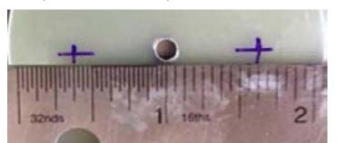
Step 2 - Stack 2 large bulkplates and 1 smaller bulkplates and temporarily secure the plates with a single eyebolt to hold them together. Drill through all 3 bulkplates at the points you just marked with a 3/16" drill bit. You can also drill a single 1/8" hole for the ematch wires.
