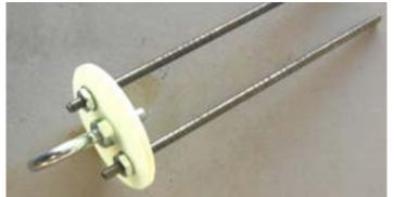
Step 4 - DO NOT EPOXY OR USE THREAD LOCK FOR THIS STEP. Place the bulkplate set with the threaded rods on one end of the long coupler. Place the other bulkplate set on the other end of the coupler and secure using a nut and washer on each threaded rods. The larger bulkplates should seat against the coupler edge with the smaller bulkplates going inside the coupler. After you are satisfied with the fit, you can remove for the next steps.
