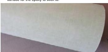
Step 11 - Sand the outside of the motor tube to rough up the surface for the epoxy to stick to.
