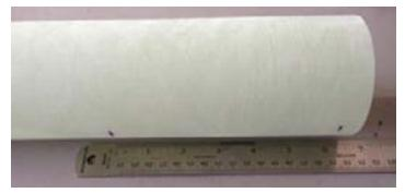
□ Step 19 - Sand the slotted main body tube for at least 1/2" around the fin slots inside and outside to rough the surface for the fin fillets. Also sand where the centering rings will attach in front of the fin slots on the inside. You can wrap sand paper around a large dowel to help sand the inside of the body tube.
