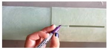
Step 2 - Use a door jamb to mark the full length of the coupler. This will help later when marking other tubes.
