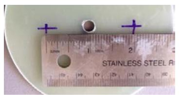
□ Step 12 - Stack the 2 large bulkplates and 2 smaller bulkplates and temporarily secure the plates with a single eyebolt to hold them together. Drill through all 4 bulkplates at the points you just marked with a 1/4" drill bit.
