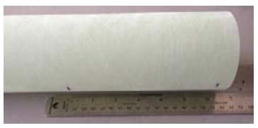
☐ Step 19 - Sand the slotted main body tube for at least 1/2" around the fin slots inside and outside to rough the surface for the fin fillets. Also sand where the centering rings will attach in front of the fin slots on the inside. You can wrap sand paper around a large dowel to help sand the inside of the body tube.
