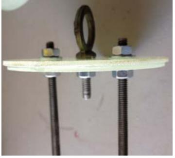
☐ Step 14 - DO NOT EPOXY OR USE THREAD LOCK FOR THIS STEP. Place the bulkplate set with the threaded rods on one end of the long coupler. Place the other bulkplate set on the other end of the coupler and secure using a nut and washer on each threaded rods. The larger bulkplates should seat against the coupler edge with the smaller bulkplates going inside the coupler. After you are satisfied with the fit, you can remove for the next steps.
