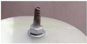
Step 5 - Epoxy the bulkplate into the end of the coupler where you sanded the inside. Leave about 3/8" for a fillet. After the epoxy sets, apply a fillet around the inside edge.
