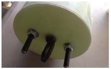
Step 15 - Mount the switch band in the center of the long coupler so 5" of coupler is exposed on each side. Place a thin layer of epoxy in the center of the coupler and slide the switch band over the epoxy while rotating so the epoxy slowly goes under the switch band. Make sure you clean up the edges of the switch band so it seats against the body tube later. After the epoxy sets, you can drill any desired altimeter vent holes and switch holes you need in the switch band.
