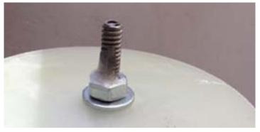
□ Step 5 - Epoxy the bulkplate into the end of the coupler where you sanded the inside. Leave about 3/8" for a fillet. After the epoxy sets, apply a fillet around the inside edge.
