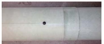
□ Step 17 - Sand the outside of the motor tube to rough up the surface for the epoxy to stick to.
