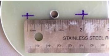
□ Step 12 - Stack the 2 large bulkplates and 2 smaller bulkplates and temporarily secure the plates with a single eyebolt to hold them together. Drill through all 4 bulkplates at the points you just marked with a 1/4" drill bit.
