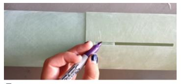
Step 2 - Use a door jamb to mark the full length of the coupler. This will help later when marking other tubes.
