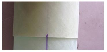
Step 9 - Measure to the middle of the payload tube and drill a single 1/8" hole for a vent hole.
