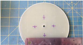
□ Step 12 - Stack the 2 large bulkplates and 2 smaller bulkplates and temporarily secure the plates with a single 1/4-20 bolt (not supplied) to hold them together. Drill through all 4 bulkplates at the points you just marked with a 5/16" drill bit.
